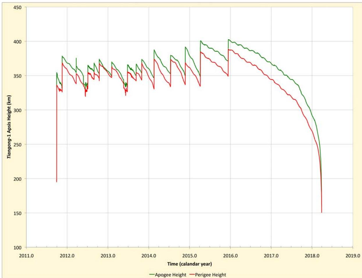
**Figure 1. As-flown apogee height (green) and perigee height (red) are plotted as functions of time for *Tiangong-1* from its day of launch until its atmospheric entry and incineration circa 2.0 April 2018 UT.**
