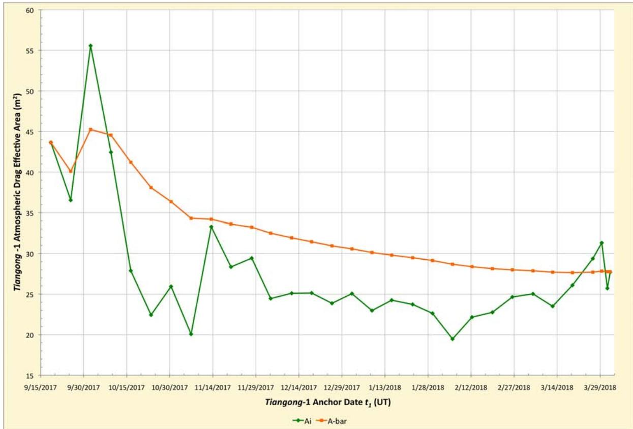
**Figure 2.** Values for  $A_i$  (green) and  $\bar{A}$  (orange) are plotted as functions of anchor date  $t_1$  as this analysis is conducted during the final half year of *Tiangong-1*'s orbit lifetime. Although the two functions must have equal values initially by definition, there is no guarantee this condition will be approached to any great precision subsequently. But such appears to be the case for the final  $A_{31}$  value with  $t_1 = 1$  April 2018 @ 11:45 UT.
