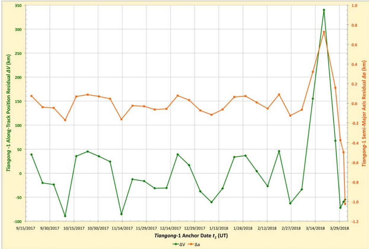
**Figure 3. Residuals associated with  $A_i$  iterations (reference Table 1's example) are plotted as functions of  $t_1$ . The along-track position residual  $\Delta V$  function and scale are colored green, while the semi-major axis residual  $\Delta a$  function and scale are colored orange. Note the null condition for  $\Delta V$  is nearly 3 horizontal grid lines below the null condition for  $\Delta a$ .**
