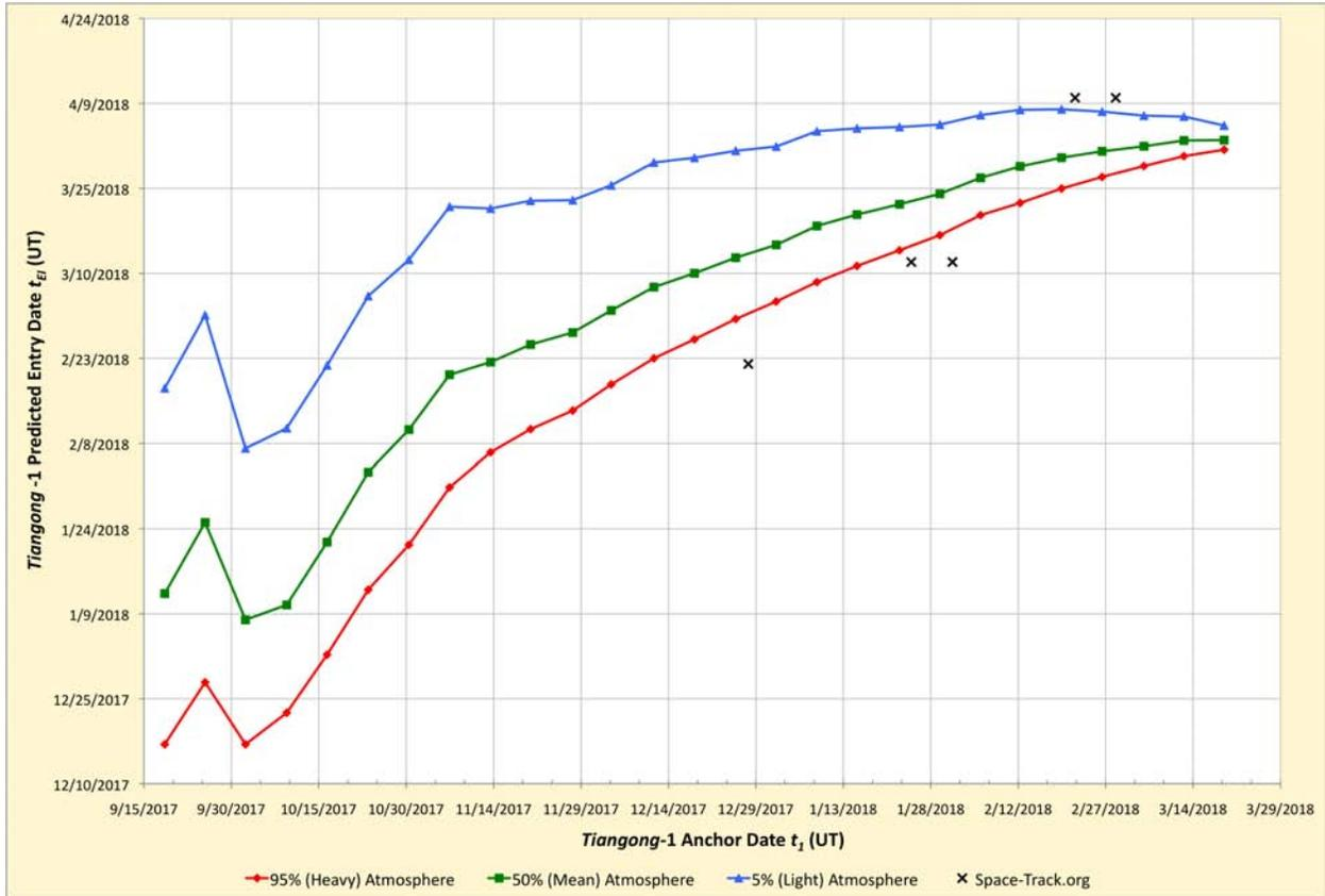
**Figure 4.** For 95% heavy (red), 50% mean (green), and 5% light (blue) atmospheres, predicted  $t_{EI}$  is plotted as a function of anchor epoch with  $t_I$  extending from 18.6 September 2017 UT to 19.3 March 2018 UT. Contemporaneous predictions posted at Space-Track.org are plotted with black "X" markers.
