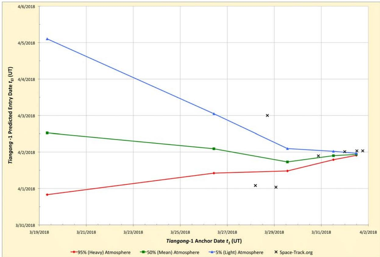
**Figure 5.** For 95% heavy (red), 50% mean (green), and 5% light (blue) atmospheres, predicted  $t_{EI}$  is plotted as a function of anchor epoch with  $t_I$  extending from 19.3 March 2018 UT to 1.5 April 2018 UT. Contemporaneous predictions posted at Space-Track.org are plotted with black "X" markers.
