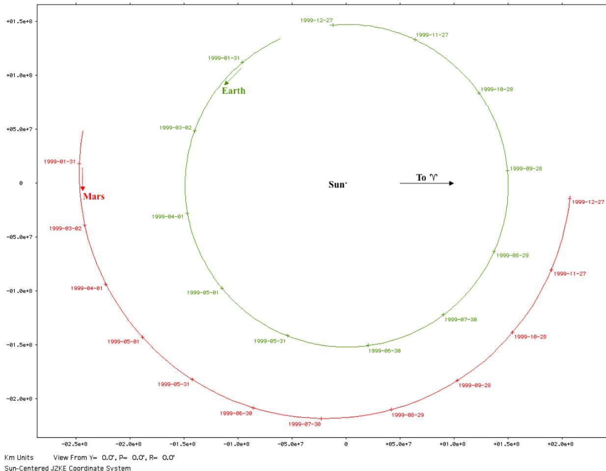
**Figure 3.** Heliocentric motion of the Earth (green) and Mars (red) is displayed with the  $x/y$  plane coincident to that of Earth's orbit, the ecliptic plane, in both Plot and Screen coordinates. At lower left, note the Plot-to-Screen transformation annotated as a null yaw-pitch-roll (Y-P-R) Euler sequence.
