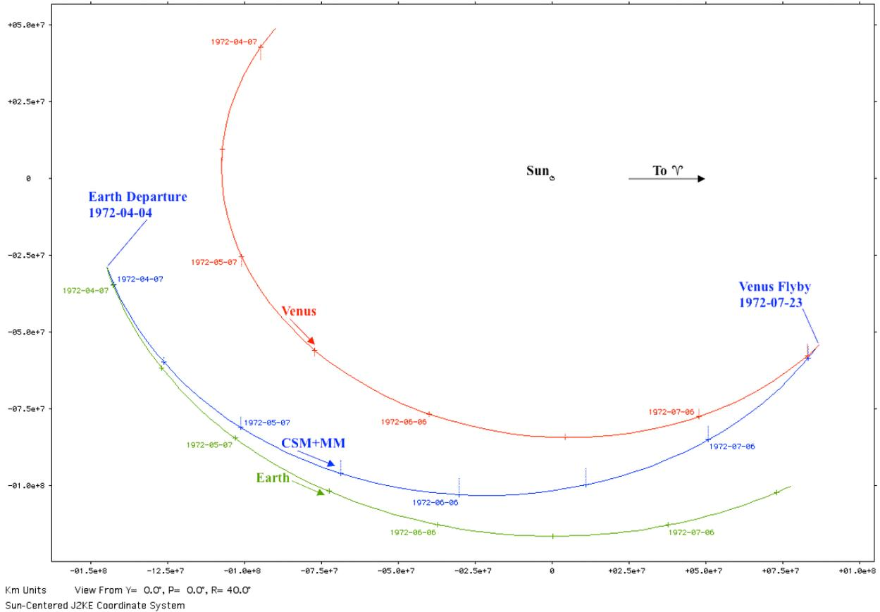
**Figure 1.** Heliocentric motion of the Earth (green), Venus (red), and CSM+MM spacecraft (blue) is plotted for Leg 1's Earth-to-Venus trajectory reproduction. The view is 40° from normal to the ecliptic plane. Date annotations are in YYYY-MM-DD format. Time ticks ("+" markers) are at 15-day intervals, and dotted lines are projections from these markers onto the ecliptic plane.
