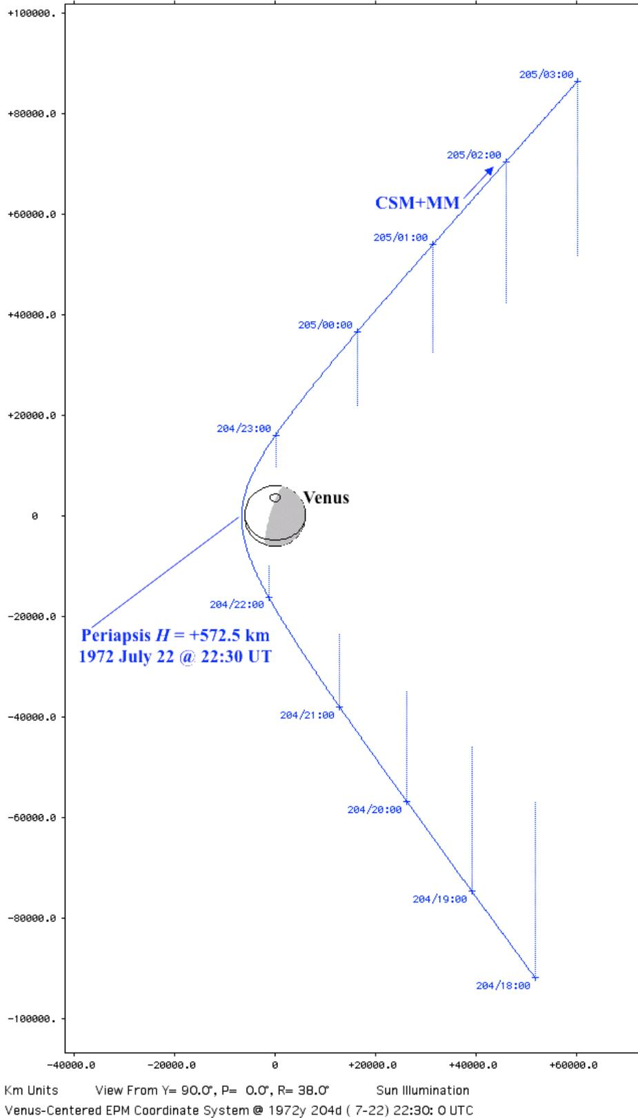
**Figure 6. Inertial Venus-centered motion of the CSM+MM is plotted during flyby. Time ticks (+ markers) are at 1-hour intervals in DOY/hh:mm format. Dotted lines are projections onto the equatorial plane of Venus, and the shaded area is the nightside of Venus.**
