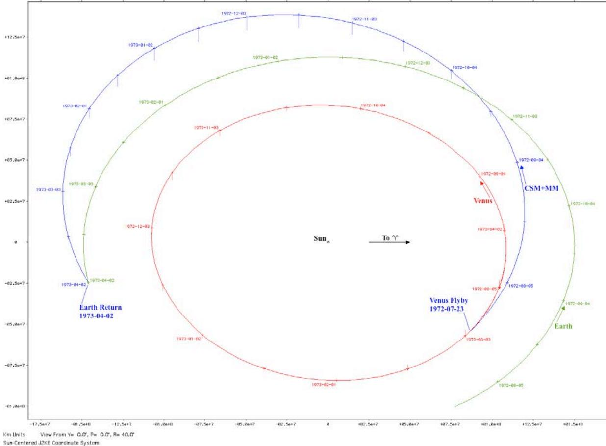
**Figure 2. Helio-centric motion of the Earth (green), Venus (red), and CSM+MM spacecraft (blue) is plotted for Leg 2's Venus-to-Earth trajectory reproduction. The view is 40° from normal to the ecliptic plane. Date annotations are in YYYY-MM-DD format. Time ticks ("+" markers) are at 15-day intervals, and dotted lines are projections from these markers onto the ecliptic plane.**
