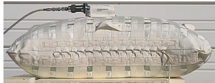
Temporary Urine and Brine Stowage System (TUBSS)
