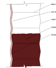
Figure 2 – Cross section of partially filled Igloo wall
