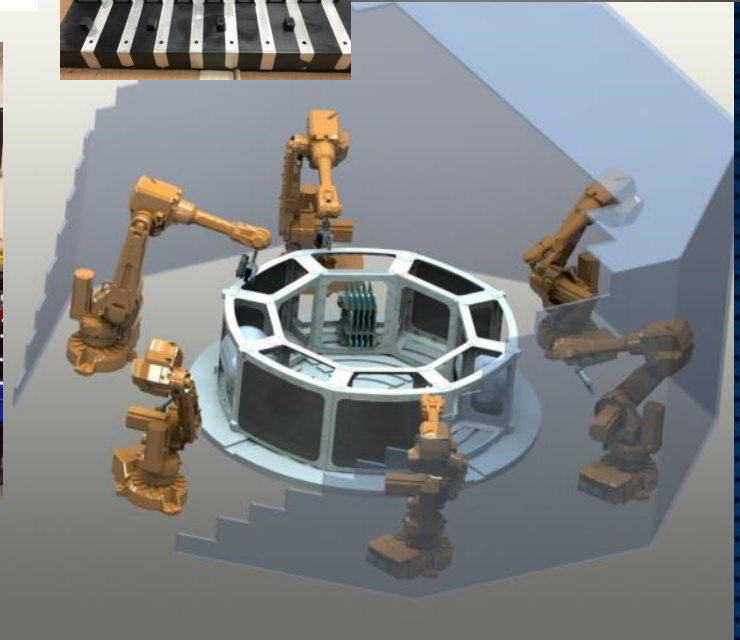
Multi-robot Additive Cluster: Additive, subtractive, fiber placement, pick and place, monitoring and inspection
