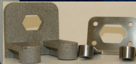
Selected Juno secondary structures built using additive manufacturing and CNT-based material
