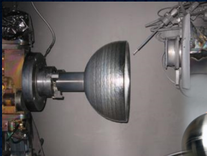
Titanium propellant tank: Additive manufacturing for schedule and cost reduction from machining forged billets
