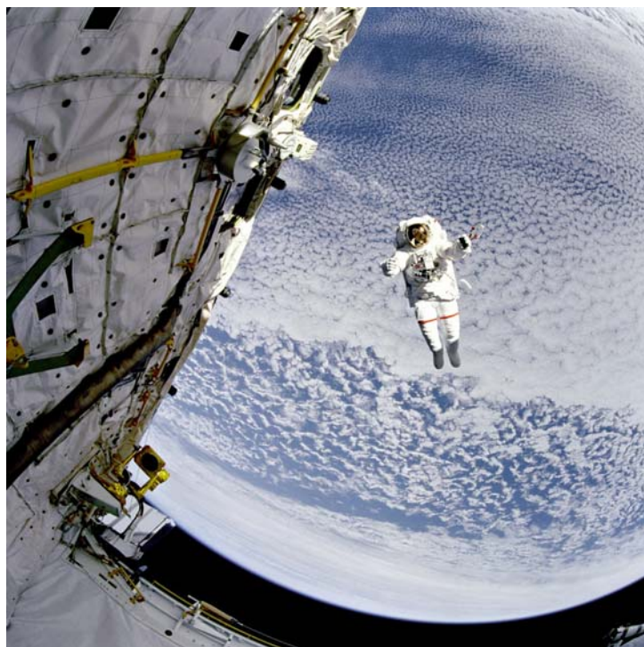
Below: Astronaut Mark C. Lee tests the new Simplified Aid for EVA Rescue (SAFER) system (NASA photo)
