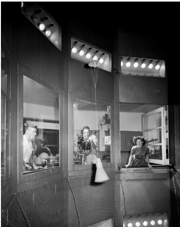
Above left: Mercury Capsule Model being tested in Langley's spin tunnel, 1959 (original photo by NACA, source: NASA)
