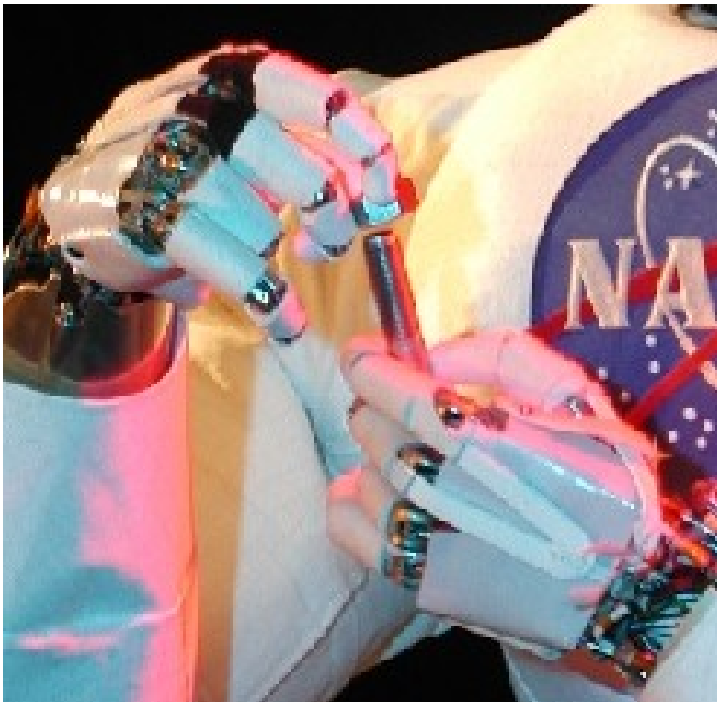
Above, : Closeup view of Robonaut's dexterous hands (NASA photo)
