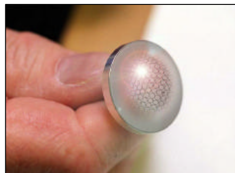
One of STARSHINE 2's 3600 1" diameter aluminum mirrors is shown here after polishing. Photo by Charlie Elms.
