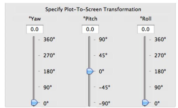
Figure 1. This user interface serves as an example of plot-to-screen transformation specification using graphic and digital input. With these null inputs, an identity transformation is invoked.
