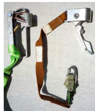
Above: Jumar ascender (left) compared to Grumman designed falling restraint (right)
