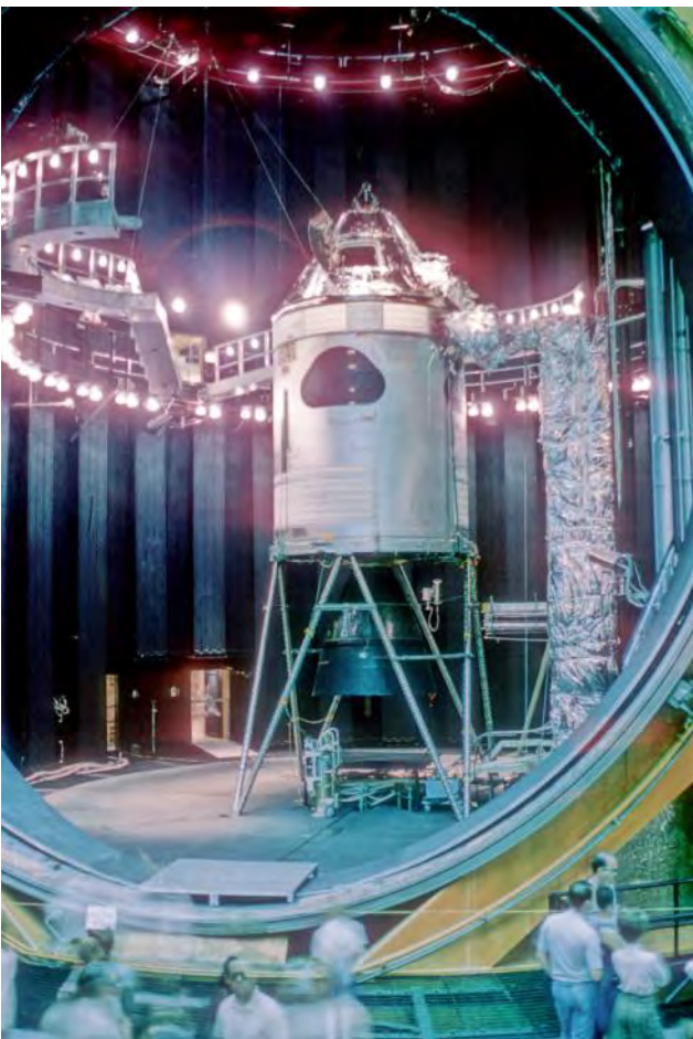
Above: a view into Chamber A through its open 40 foot diameter door. An Apollo Command and Service Module is mounted vertically. Astronauts Joe Kerwin, Vance Brand and Joe Engle spent about a week living inside the 2 TV-1 spacecraft while the chamber provided the high vacuum and severe thermal loads expected during the mission. The tests were supported by contractor personnel from Rockwell.
