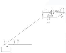
Given a ground station tracking an airplane, moving in a straight line at a constant speed, with only bearing measurements, we are interested in knowing the speed of the airplane and its position at the beginning of the tracking pass ( $x_0$ ,  $y_0$ ,  $u_0$ ,  $v_0$ ). The equations are
