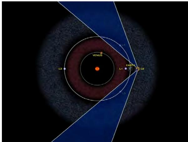
**Figure 2:** A depiction of the field(s)-of-regard of a space-based NEO survey telescope at SEL<sub>2</sub>. Such a telescope looks at the ‘sweet spots’ to find human-accessible NEOs (NASA GSFC).
