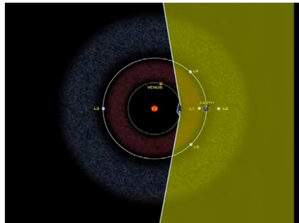
**Figure 3:** Field-of-regard for a space-based NEO survey in a Venus-like orbit. Such an orbit is geometrically optimized to locate NEOs at opposition when they are brightest, even those interior to Earth's orbit. (NASA GSFC).
