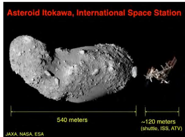
**Figure 8:** Comparative size of asteroid 25143 Itokawa and the ISS (with shuttle and ATV) to scale. Rendezvous and proximity operations in and about the ISS are akin to that of visiting NEOs. Due to their inconsequential gravity wells, spacecraft must station keep in proximity to the small body. Unlike flybys, it is necessary to stay at the asteroid to survey and characterize it with robotic precursors prior to human visits (JAXA, NASA, ESA).
