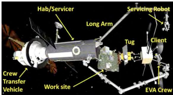
**Figure 13:** (from left to right) Crewed vehicle, Hab/servicing module with attached worksite, and space tug/grapple. Servicing in GEO may very well be the key stepping stone to planetary deep space destinations such as NEOs (NASA JSC).
