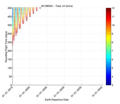
Figure 3. The 2013 BS<sub>45</sub> PCC posted 20 February 2013 at the NHATS website shows viable mission opportunities on the wane at the earliest NHATS-compliant Earth departure dates during year 2015. In accord with the  $\Delta v_{TOT}$  color legend at right, a NEO with ideal HSF accessibility would sport deep blue pixels at any programmatically desirable Earth departure date with minimum roundtrip flight time.
