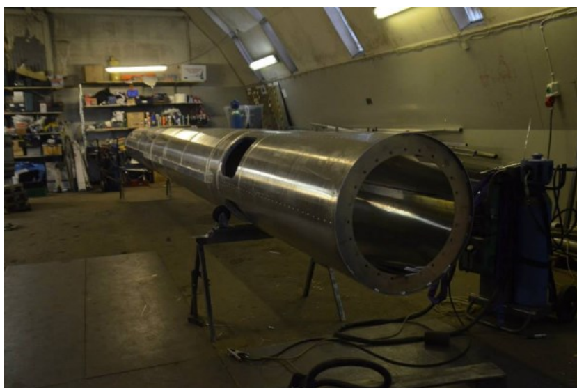
Above: The tubes to contain the chambers for fuel and oxidizer. Image credit: Shen Ge.
