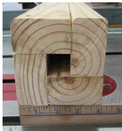
Above: Four pieces of wood making the pedestal to wrap around the pipe. Image credit: Jim Wessel.
