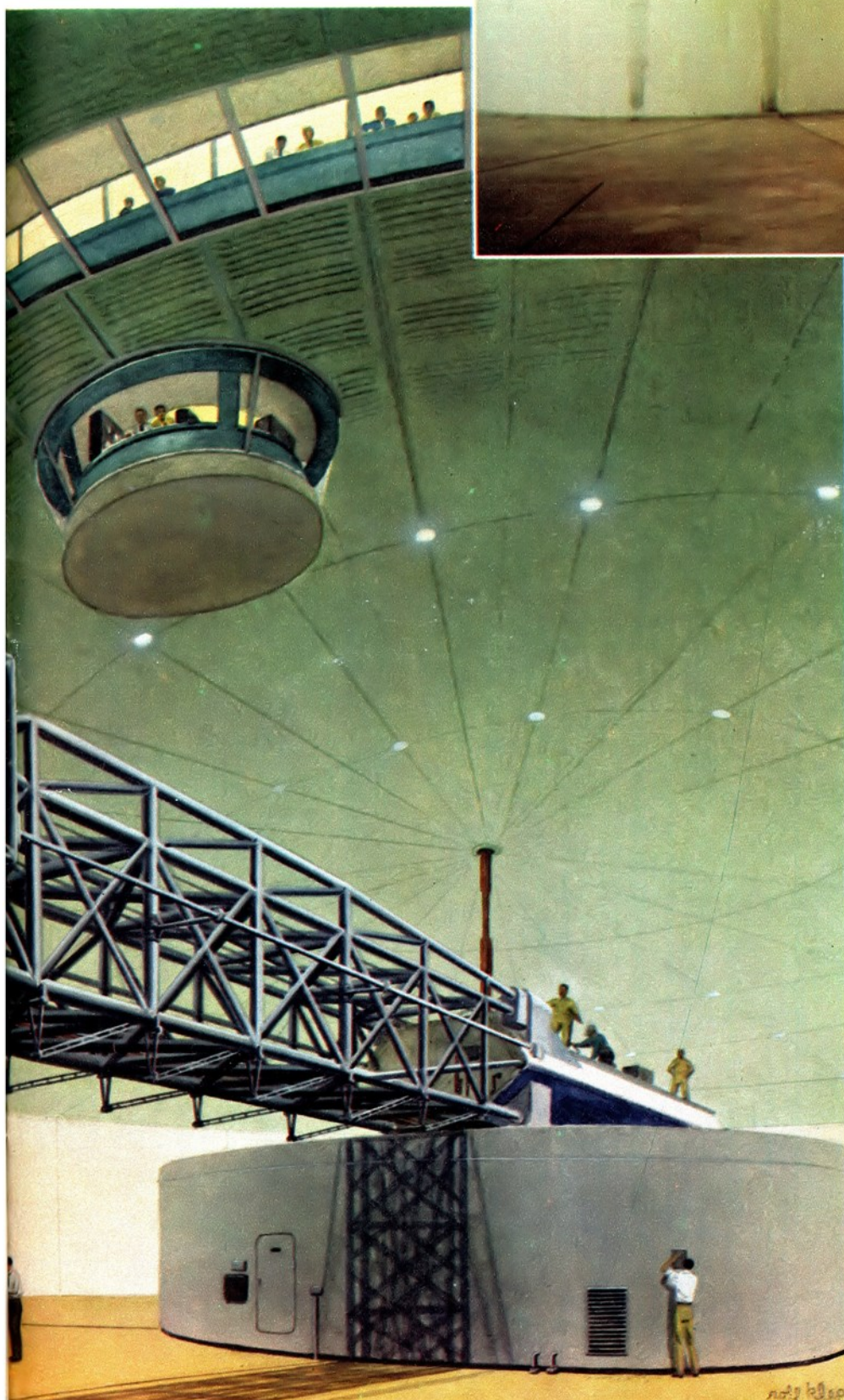
Navy centrifuge at Johnsville, Pa., one of several in use to simulate acceleration force
