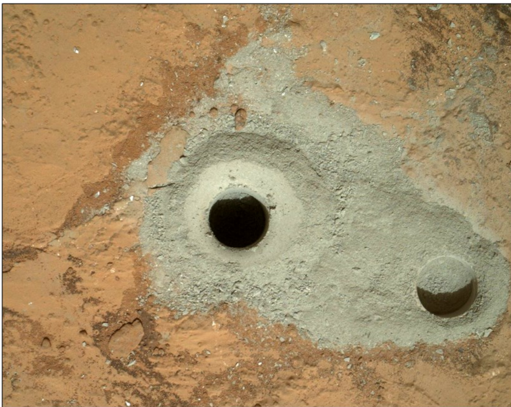
Fig. 9. Curiosity's first sample drilling. At the center of this image is the hole in a rock called "John Klein" where Curiosity conducted its first sample drilling on Mars. The drilling took place on February 8, 2013, or Sol 182, Curiosity's 182nd Martian day of operations. A preparatory, test shallower hole (the one on the right) was drilled two days earlier, but the deeper hole resulted from the first use of the drill for rock sample collection. The image was obtained by Curiosity's MAHLI camera on Sol 182. The sample-collection hole is 0.63 inch (1.6 centimeters) in diameter and 2.5 inches (6.4 centimeters) deep. The "mini drill" test hole near it is the same diameter, with a depth of 0.8 inch (2 centimeters). Image credit : NASA/JPL-Caltech/MSSS.
