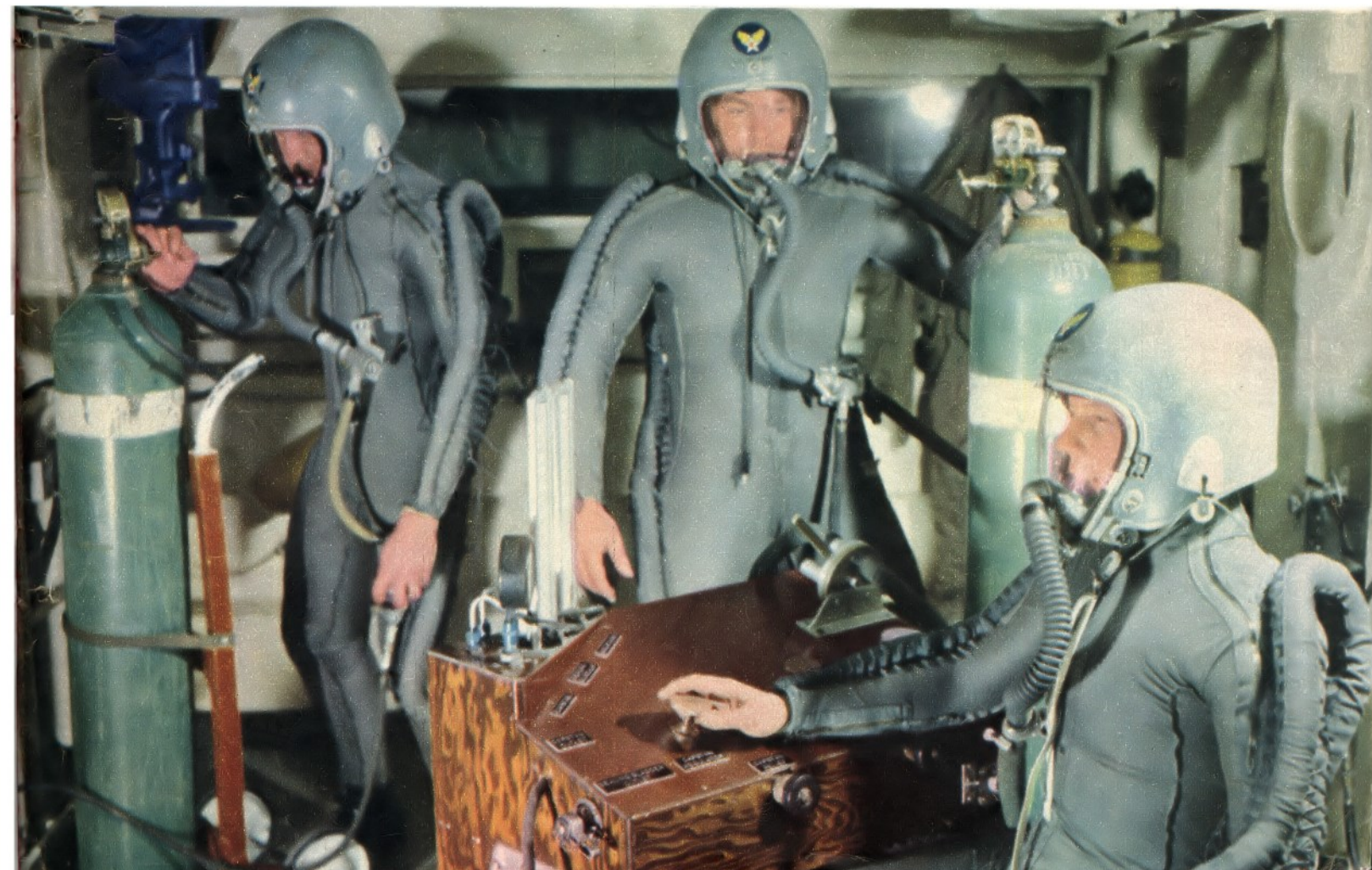
New Navy space suit is a one-piece affair, with helmet hinged to the shoulders. It has been tested to altitudes of 63,000 feet and still higher tests are under way. Many details of the suit are top secret
