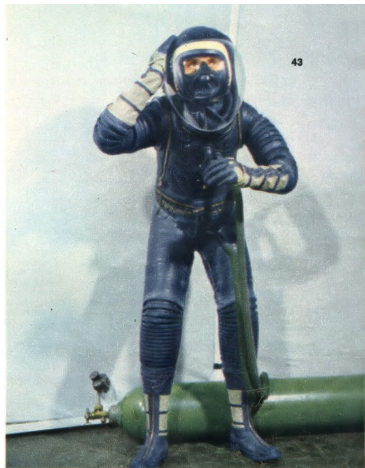
Suit permits great freedom of movement. It was designed by Carroll P. Krupp, of Findlay, O., 35-year-old self-taught Goodrich engineer, under the direction of U.S. Navy's technicians. It would work on the moon
