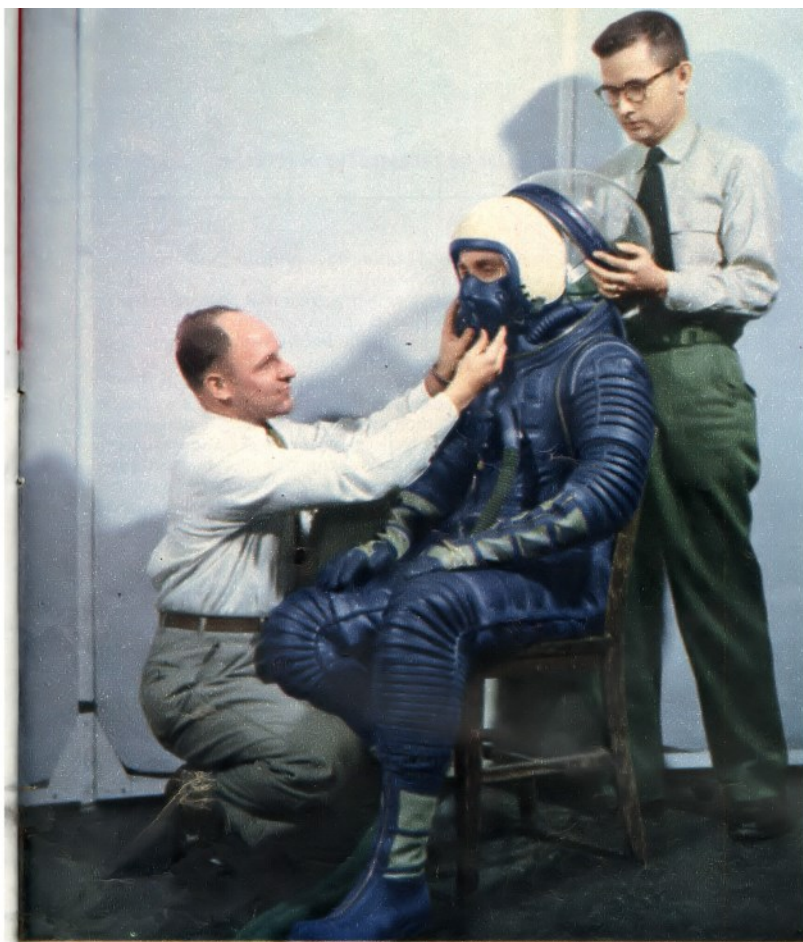
New Navy space suit is a one-piece affair, with helmet hinged to the shoulders. It has been tested to altitudes of 63,000 feet and still higher tests are under way. Many details of the suit are top secret
