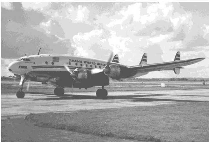
Above: Lockheed L-749A Constellation N6022C "Star of Virginia" TWA at London (Heathrow) Airport with under-fuselage "Speedpack" freight container. September 12, 1954. Image source: Wikipedia. Image credit : RuthAS.
