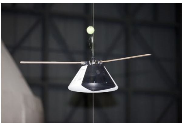
Above: A model capsule seen ahead of drop tests inside the Vehicle Assembly Building at NASA's Kennedy Space Center in Florida to test a rotor system landing design. Image credit: NASA/Kim Shiflett.
