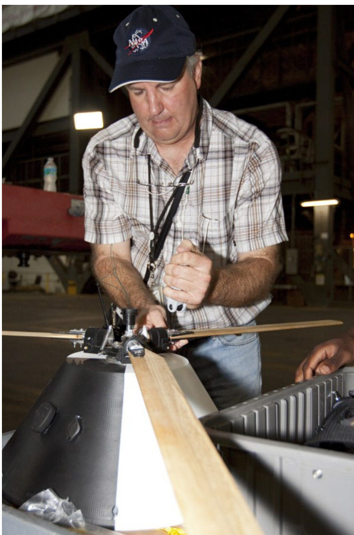
Above: NASA's Johnson Space Center Aerospace Engineer Jeff Hagen attaches a rotor to the top of a model capsule ahead of drop tests inside the Vehicle Assembly Building at NASA's Kennedy Space Center in Florida. Image credit: NASA/Kim Shiflett.
