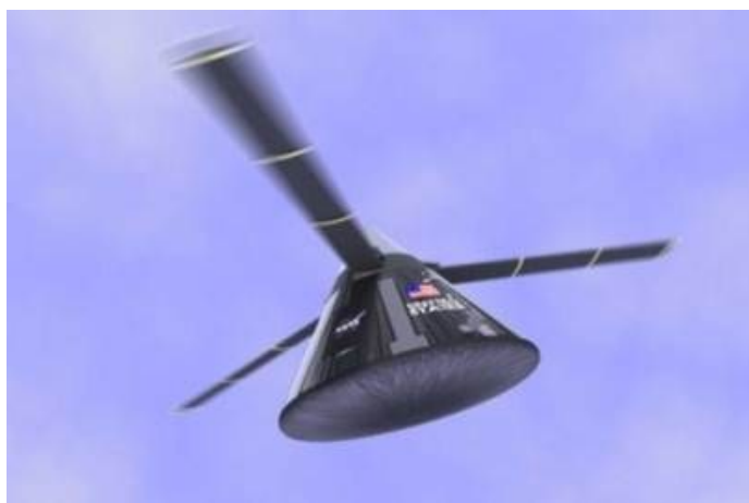
Above: An artist concept shows a capsule flying back to Earth with a rotor blade system instead of parachutes. The rotors deploy from the side of the capsule once the fall has slowed to subsonic speeds. Image credit: NASA.
