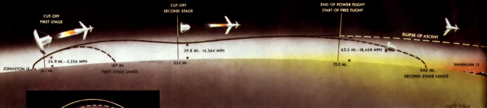
Contrary to widespread notion, rocket ship does not travel straight up all the way. After covering first eight miles vertically, rocket proceeds at angle. Inset art shows complete flight path into two-hour orbit; section in rectangle marks flight segment detailed above
