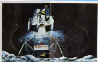
11 With descent stage as a launch pad, the ascent stage fires for liftoff.
