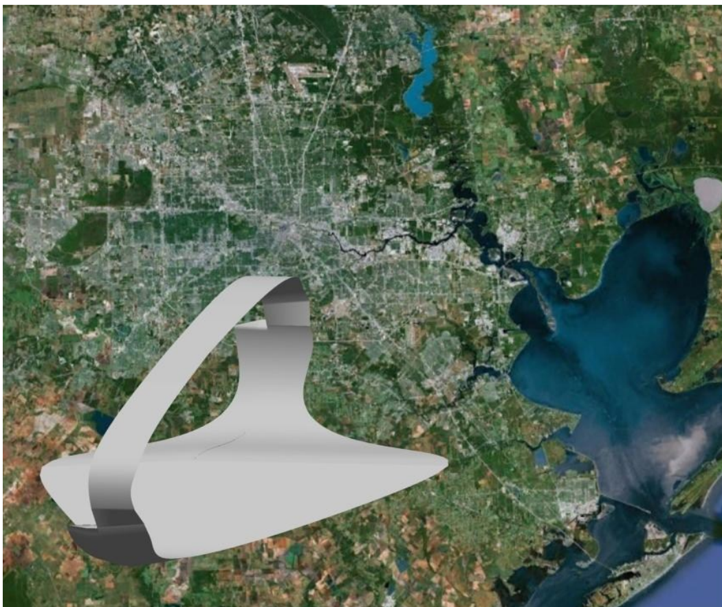
Figure 2. A Ring Wing Waverider (RWWR) vehicle. Image credit: Dr. Patrick Rodi.
